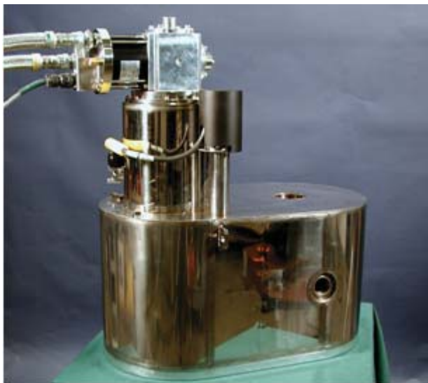
Radial access RTB magnet system
